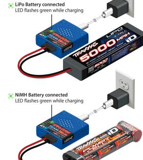
Note: It is normal for the charger to become warm while charging at the maximum charge rate. If the charger is not in a cool, well-ventilated area, the charge rate will be automatically reduced to prevent the charger from overheating.
